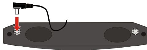
Figure 14 Connect External Power Supply
