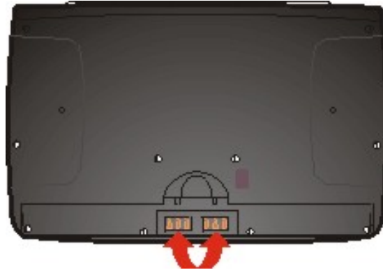
Figure 8 Battery Contacts in Battery Compartment
