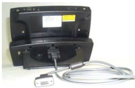
Figure 38 ActiveSync Cable Connected to Serial port on Cradle
